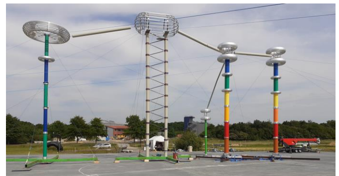
Fig. 7 Open area test site at PTB, high-voltage generator for 2000 kV DC (centre) and four precision voltage dividers for high DC voltages
